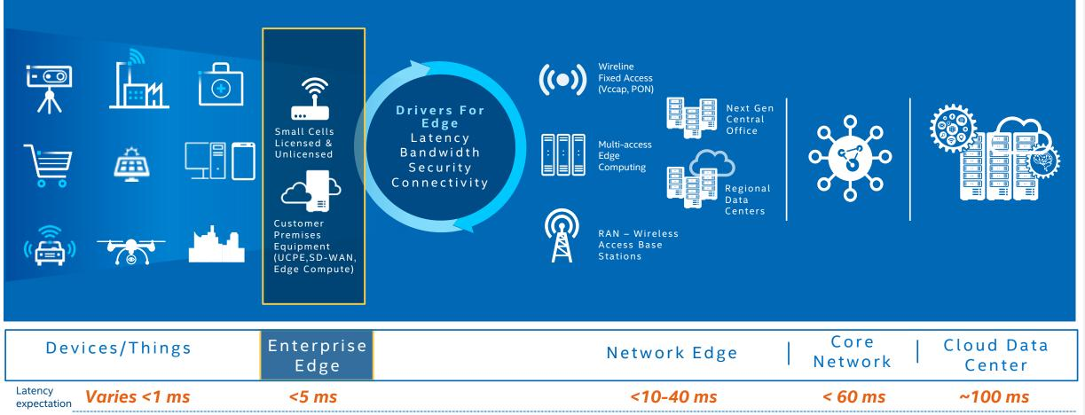
Flexibility to run workloads on-prem, at the network edge, or in the data center/cloud. Enable low latency apps, e.g. Power backbone disconnect (<4ms), high speed machinery cut-off (1ms), Surveillance camera feed analysis (2ms)
