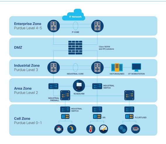
**Industrial** - Level 0 - Field: Sensors, actuators, motors
