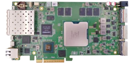
Intel NetSec Accelerator Reference Design Ver 2 (Intel® Xeon® D: 4C, 8C, 10C)
