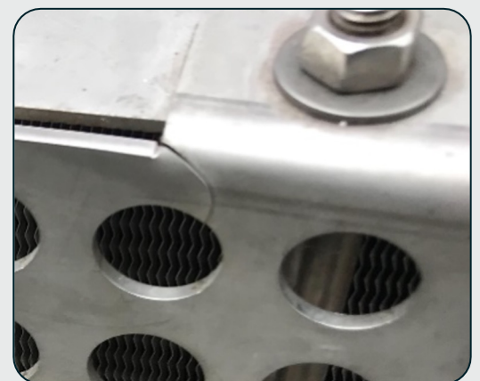
Cracks on the cooling bundle
