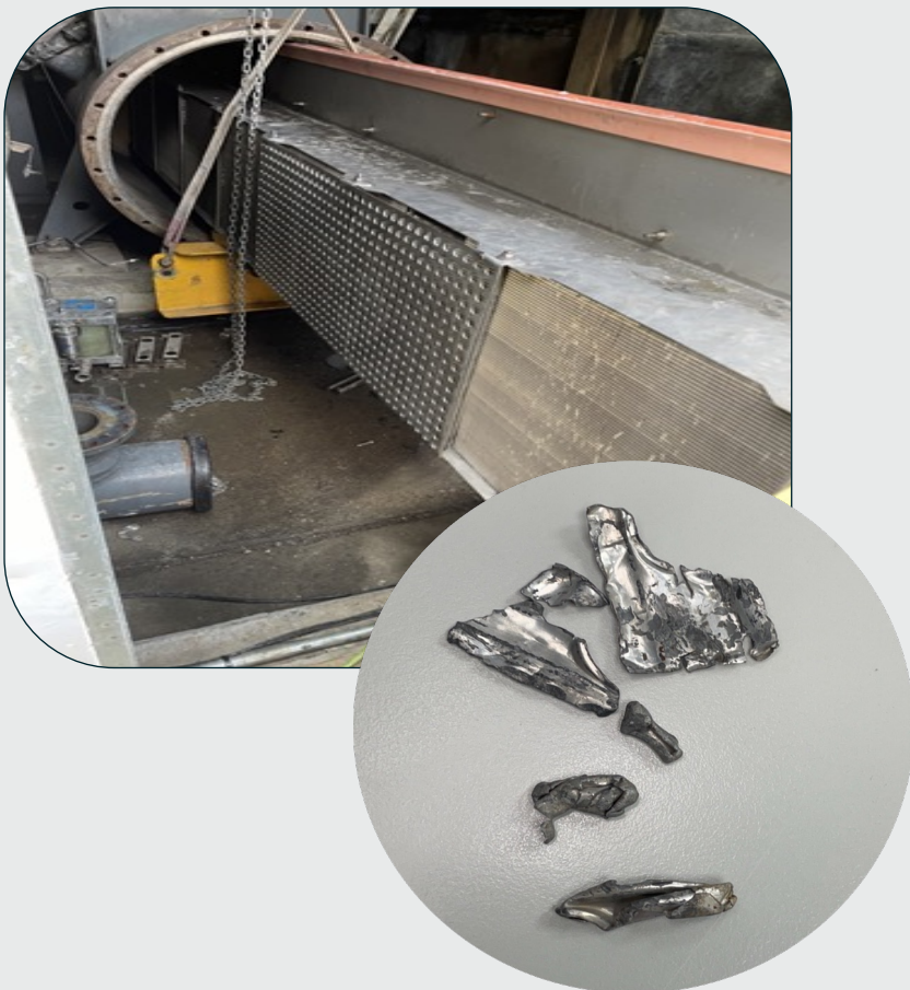
Pieces of aluminum from the cooling fin
